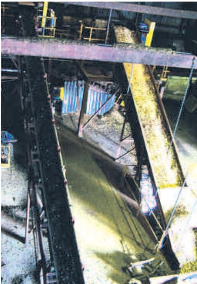
Tire-derived fuel is delivered pre-shredded and travels on a conveyor (left) at a speed that appropriately mixes TDF with waste wood from the conveyor at right just before entering the boiler.
